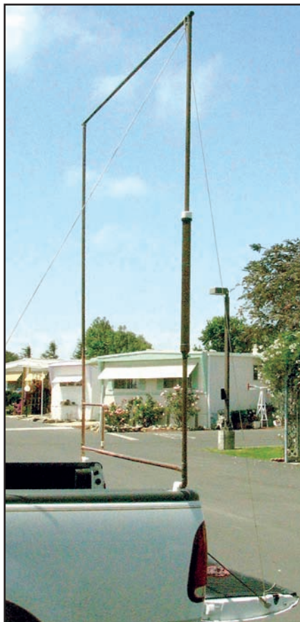
Figure 3 — The loop mounted on the bed of the author's ¾ ton long bed pickup.
